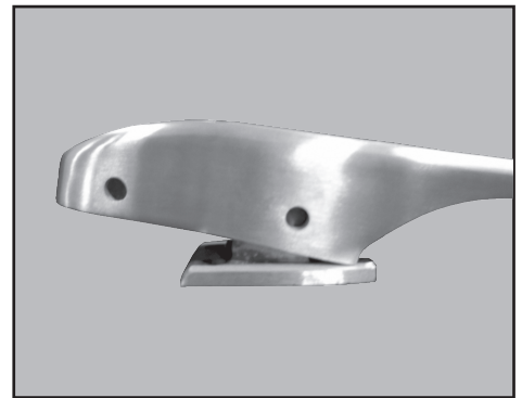
3. Place handle over base, lining up side holes of handle with side holes of base. Note: Handle will resist due to spring tension as it's forced down. Make sure opposite end of spring has engaged handle boss.
